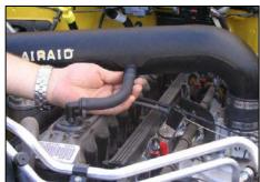
**26.** Connect the other end of the valve cover hose to the intake tube. Secure both ends of the hose using the supplied black speed clamps.
