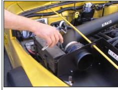
**24.** Make final adjustments to the intake tube for correct position. Tighten all four hose clamps and bracket bolt.
