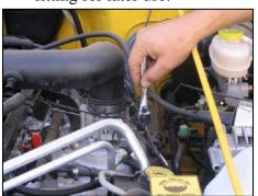
Loosen hose clamps on both ends of factory intake tube. Remove intake tube from engine.
