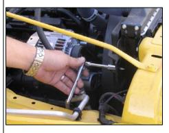
**6.** Using a 7/16" socket, remove the factory radiator mount bolt. Retain bolt for later use.
