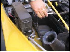
5. Using a 5/16" socket, remove the three nuts and bolts mounting the factory air filter housing to inner fender.
