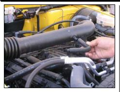
1. Disconnect negative battery cable. Remove factory valve cover breather hose from intake tube and discard. Retain plastic valve cover fitting for later use.
