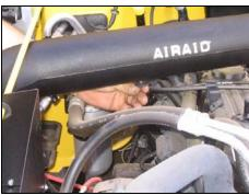
**23.** Mount the Airaid intake tube to the valve cover bracket using the supplied <sup>1</sup>/<sub>4</sub>" bolt and washer as shown above.
