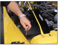
**14.** Using the supplied ½ x 20 nut, bolt and washers, mount the front of the Airaid Cool Air Dam to the inner fender.
