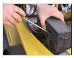
7. Using a flat blade screwdriver, push locking tabs inward to remove the fuse panel from the mounting bracket.
