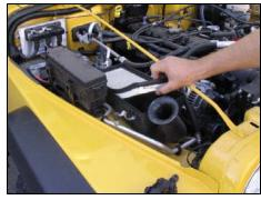
**4.** Remove factory air filter from air box.
