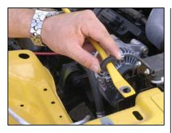
**11.** Using the supplied thin grommet, position it over the passenger side radiator support rod as shown above.
