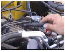
**19.** Install the supplied rubber hose on the factory plastic valve cover breather fitting.
