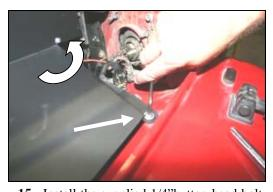
**15.** Install the supplied 1/4"button head bolt (#11), and 1/4" washer (#12), thru the CAD, with the 1/4" fender washer (#13) and nut (#14), on the bottom of the fender. Re-install the factory bolt in the radiator shroud removed in step #9.
