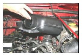
**6.** Remove the resonator from the vehicle.
