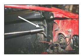
**9.** Remove one bolt from the passenger side radiator fan shroud and save it for step #15.
