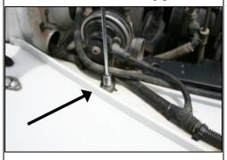
**5.** Using a 10mm socket, remove the horn bolt. (Save for later use.)
