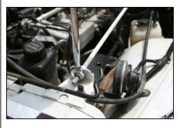
**8.** Using a 9/16" wrench, loosen the nut on the radiator rod support, and lift it up.
