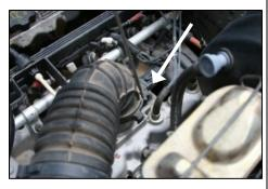
**3.** Pry open the plastic clamp that holds the factory intake tube to the throttle body. Unhook the 3 metal latches on the airbox that hold it to the mounting plate, and remove the intake assembly.
