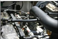
17. Replace the factory breather hose with ½"x10" rubber hose between valve cover and intake tube using speed clamps as shown.
