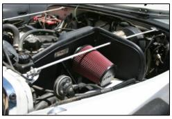
**18.** Install the Airaid Premium Filter and the weather strip on the **CAD**, as shown. (Hint: start the weather strip near the radiator support and work towards the back of the vehicle.)
