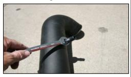
**14.** Install the ¼" barbed fitting into the intake tube.
