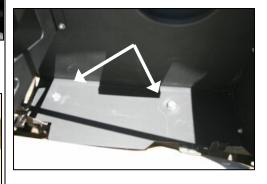
**10.** Install two ¼"-20 bolts and washers thru the top, and fender washers and nuts on the bottom, where the factory grommets were removed.
