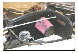
**18.** Install the Airaid Premium Filter (#1) and the weather strip (#9) onto the **CAD**, as shown. (Hint: start the weather strip near the radiator support and work towards the back of the vehicle.)
