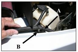
**12.** A) Using a <sup>1</sup>/<sub>4</sub>-20 bolt (#13), 2 washers (#14), and locknut (#16), bolt the CAD to the fender. B) Install the wire loom clamp into the hole in the **CAD**, as shown.
