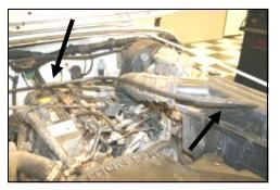
1. <u>Disconnect the negative battery cable.</u> Remove the factory valve cover breather hose from the airbox , and the valve cover.
