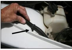
**6.** Carefully remove the wire loom clamp from the hole in the inner fender. Use caution not to damage the clamp, as it will be reused.
