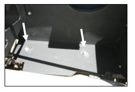
10. Install two  $\frac{1}{4}$  - 20 x 5/8" hex bolts (#13) and 1/4" flat washers (#14) thru the top of the **CAD**, and fender washers (#15) and locknuts (#16) on the bottom, where the factory grommets were removed.
