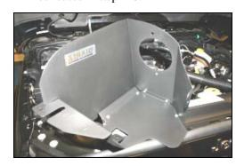
**11.** Assemble the Cool Air Dam panels (#3 & 4) as shown, using the seven 6-32 screws (#10), flat washers (#11), and keps nuts (#12).
