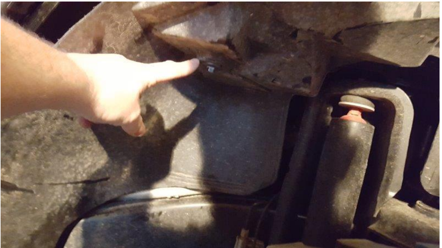
34. Using wire cutters, cut the 2 wires at the base of the factory side marker lamp.
