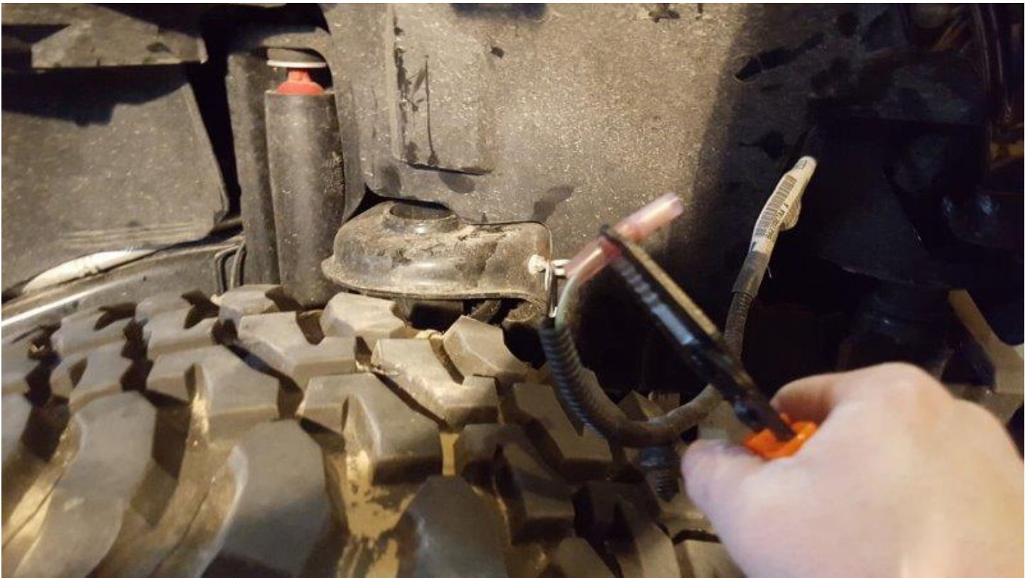
37. Using heat gun (hair dryer works also but takes longer) seal the heat shrink tubing around each wire.
