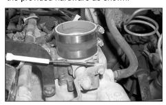
16. Install the provided silicone hose and hose clamps onto the throttle body as shown.
