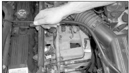
2. Disconnect the crank case vent hose.
