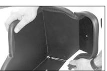
10. Apply the provided trim seal to the heat shield as shown and trim if necessary.
