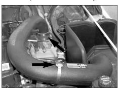
17. Install the K&N intake tube into the silicone hose and line up the other end of the tube with the saddle bracket, then secure the tube to the throttle body and the saddle bracket with the provided hose clamp.
