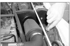
22. Install the K&N Filtercharger onto the K&N intake tube and secure with the provided hose clamp as shown.
