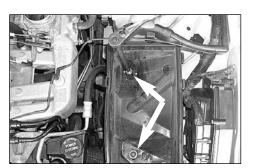
6. Loosen and remove the two bolts that secure the lower air cleaner assembly, then remove lower airbox from vehicle.
