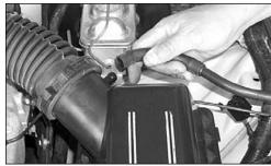
3. Remove the EVAP canister vent line from the air cleaner lid
