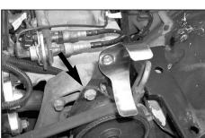
9. Using the bolt removed in step 5, secure the saddle bracket assembly to the alternator as shown, but do not tighten completely at this time.
