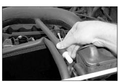
21. Connect the hose to the vent on the K&N intake tube, then, connect the other end to the EVAP canister vent line as shown.
