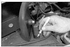
14. Install the bracket onto the K&N heat shield and line up the bracket with the inner fender then mark the hole and drill a  $\frac{1}{4}$ " hole.
