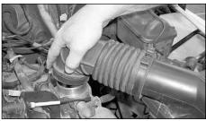
4. Loosen the hose clamp at the throttle body, then detach the stock intake tube from the throttle body as shown.
