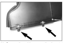
11. Secure the rubber mounting inserts to the holes on the heat shield with the provided bolts and washer. But do not tighten.
