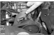
7. Remove the upper power steering pivot bolt as shown.
