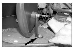
15. Secure the "L" bracket to the fender using the provided hardware as shown.
