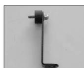
13. Assemble the "L" bracket and the rubber mounted stud using the provided hardware as shown.
