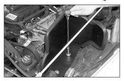
12. Install the heat shield and insert the rubber mounting inserts into the stock air cleaner locating holes and tighten as shown.
