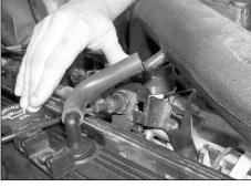
19. Install the 5 inch hose onto the crankcase vent, then connect the other end to the vent on the K&N intake tube as shown.
