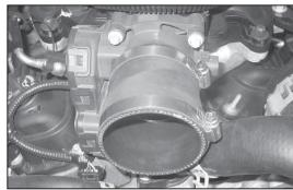
9. Install the supplied silicone hose (08096) onto the throttle body and secure with the supplied hose clamp.
