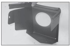
13. Install the supplied edge trim onto the heat shield as shown.
