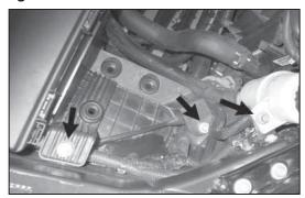
12. Remove the power steering reservoir mounting bolt and the two airbox bracket mounting bolts shown.
