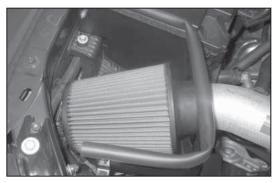
21. Install the K&N® air filter and secure with the provided hose clamp.
