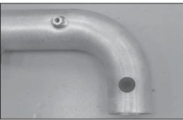
6. Install the supplied grommet into the hole in the  $K\&N^{\otimes}$  intake tube as shown.
