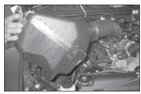
5. Lift up the airbox assembly to dislodge it from the mounting grommets and remove the complete assembly from the vehicle.
