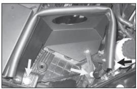
18. Install the heat shield assembly into the engine compartment and secure with the three bolts removed in step #12.
