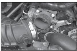
4. Loosen the hose clamp that secures the stock intake tube to the throttle body and then disconnect the intake tube from the throttle body.
