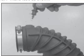
7. Remove the air temperature sensor from the stock intake tube as shown.
