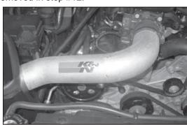
19. Insert the K&N® intake tube into the silicone hose at the throttle body and align with the mounting bracket installed in step #11 and then secure with the hose clamp and hardware provided.
