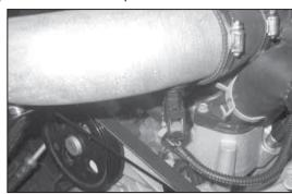
22. Reconnect the air temperature sensor electrical connection.
