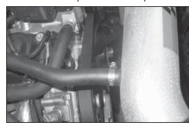
20. Connect the crankcase vent hose to the K&N® intake tube and secure with the provided hose clamp as shown.
