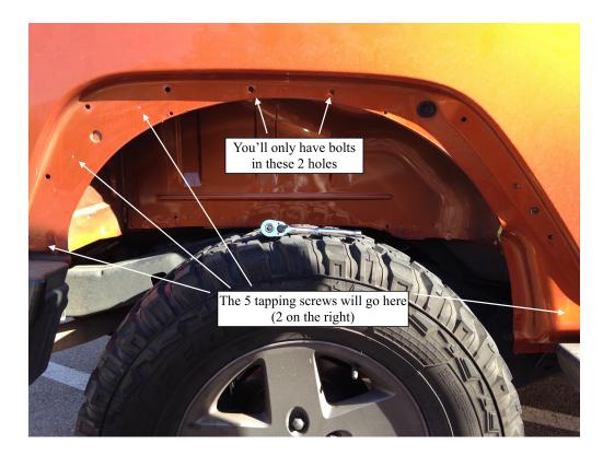
6. Place new flare against the body aligning the holes. Loosely place (2) of the 10mm bolts with (4) washers and (2) nuts. Once in place, go back and tighten all bolts. Use the mounting holes on the new flare as guides for the (5) tapping screws.
