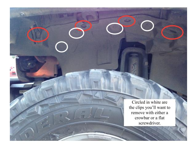
2. Be sure to disconnect the front turning signal plug, just twist and pull. Next, start pulling the fender flare towards you from front to back. You'll hear loud cracking/popping noises (this is normal), those are the clips breaking (they are disposable). Once off, tuck and secure away the turning signal wire from any interference.
