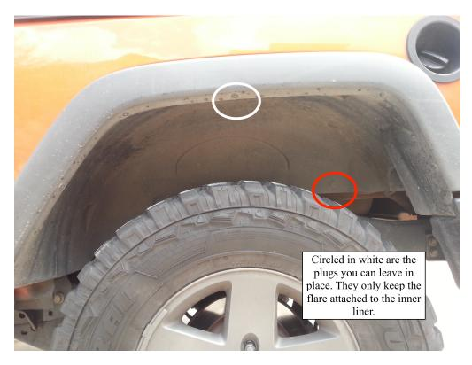
5. Like Step 2, start pulling the fender flare towards you from front to back. You'll hear loud cracking/ popping noises (this is normal), those are the clips breaking (they are disposable).
