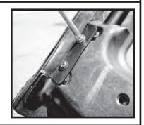
Step 6. With the assistance of a second person, raise the top and bow assembly in the up position. Lock the header to the windshield. Carefully drape the top over the windshield onto the hood. With the top portion of the header exposed remove all of the screws from the top side of the header. Remove the top portion of the header. Remove the old top from the header.
