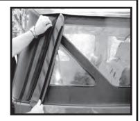
Step 13. Secure the top above the doors by inserting the plastic retainer strips into the door surround. Your new top installation is now complete.
