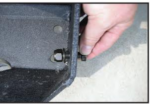
2. Insert a M12 hex bolt and washer thru the top holes in the stubby end. Install the stubby end onto the bumper by sliding the notch cutout on the lower portion of the end onto the bottom bolt. Line up the top bolts with the bumper and insert them into the bumper fastening with a hex nut and washer. Tighten all bolts. Repeat for opposite side.
