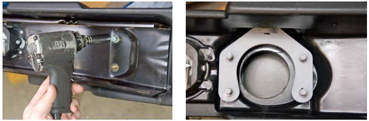
9. Find the driver side winch plate bracket. Install the bracket, using the 9/16" x 1.5" bolt, flat washer, and nut. Hand tighten at this time. Repeat on the passengers side. See Photo 7 & 8.
