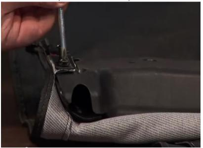
**b.** Slide the side bow (Pivot Knuckle faces in) into the opening and align the holes. Use the #8 screws provided to screw the side bow in.
