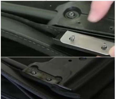
**e.** Use the foam seams to cover the metal plate. Install the foam tape strips on the front edge of the sunrider top. Foam seals have a cutout that should face the bow and a notch for the tab on the side of the top. Repeat for both sides.
