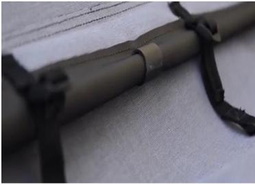
b. Pull the middle bow into position and move the rest of the fabric assembly to the back.
