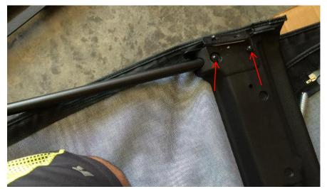
**c.** Turn the side bow over and screw the two more screws. (Its 4 screws per bow. Screws are on top and bottom of the bow). Repeat for both sides.
