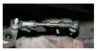
**Note:** We recommend using the "neutral" position of the transfer case as the starting point. Put the shift lever in the neutral position as well as the transfer case. Adjust the linkage accordingly.
