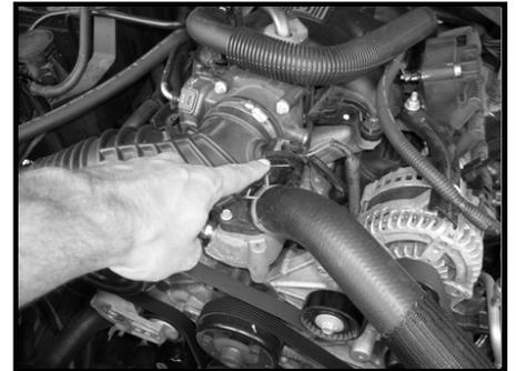
2. Loosen the 4, 8mm, bolts holding the throttle body to the intake manifold. Remove throttle body.
