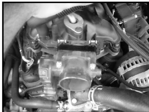
6. Reconnect electrical connector to the bottom of the throttle body; install the air inlet tube followed by the air intake temperature sensor.
