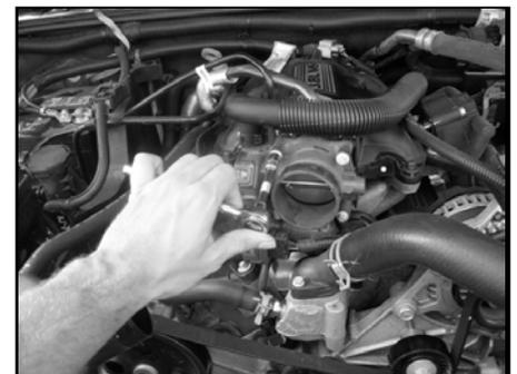
3. Disconnect the electrical connector from the bottom of the throttle body.
