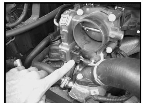
4. Place the gasket on the backside of the throttle body followed by the spacer (Logo up, rounded edge to the right). Place the supplied M6 bolts and washers through the front of the throttle body going through both the gasket and throttle body spacer.
