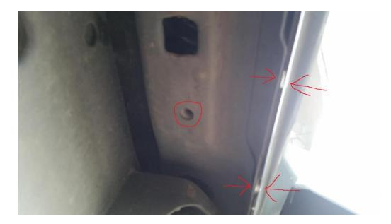
3.) Mount the bracket to the pinch weld area of the body with (2) 6mm x 25mm Button Head Allen Bolts, (4) 6mm Inside Diameter x 18mm Outside Diameter Flat Washers, and (2) 6mm Inside Diameter Nylon Lock Nuts. While holding the provided 4mm Allen Wrench on the head of the Allen Head Bolt, use a 10mm Wrench or a 10mm Socket and Ratchet to fasten the 6mm Inside Diameter Lock Nuts to the threads of the Allen Head Bolts. <u>LEAVE ALL HARDWARE LOOSE</u> <u>UNTILL STEP IS INSTALLED ONTO BRACKETS</u>,
