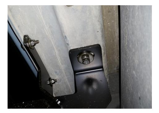
5.) Follow steps 1-4 to mount the Passenger Side Center bracket "PC", which is etched in the metal and the Passenger Rear "PR" Bracket.
