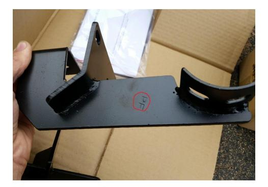
2.) Once the correct bracket has been found, locate the Passenger Front 8mm Bolt hole. Also locate the 6mm Bolt holes in the pinch weld of the body.
