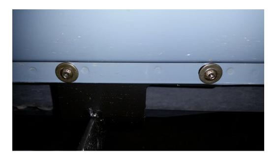
4.) Using (1) 8mm x 35mm Hex Head Bolt, (1) 8mm Lock Washer, and (1) 8mm x 28mm Outside Diameter x 3mm Large Flat Washers mount the bracket to the bottom of the body panel. Start to thread the bolt into the hole in the body panel by hand, then loosely tighten the bolt with a 13mm socket and ratchet.
