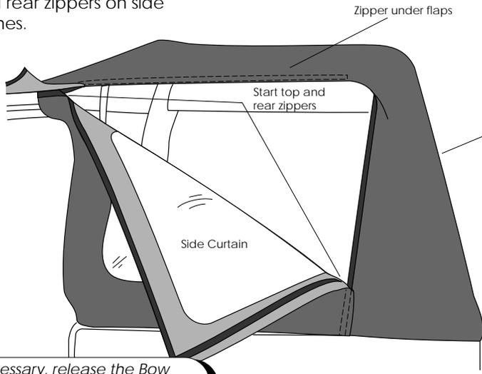
**Note:** If necessary, release the Bow Coupler and slide the top around the Corner Belt Rail towards the window to make it easier to start the zippers on the Side Curtains.
