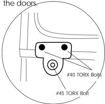
**Wrangler/YJ Windshield Adjustment:** If necessary, loosen the #40 TORX bolts in the windshield clamps to loosen the windshield in order to slip the bracket under the horizontal tube.
