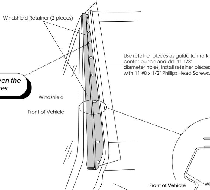
**Warning: A loose Windshield Retainer may allow the top to disengage from the windshield, causing damage to the top and possible injury to the occupants of the vehicle.**
