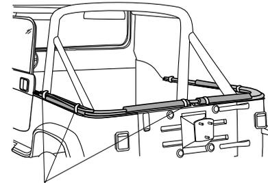
Leave packing tape on Bow Assemblies until front holes of Bow Mounts are secure
