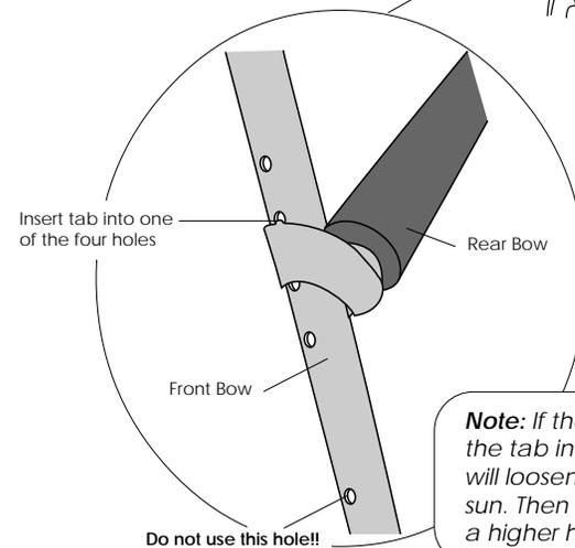
**Note:** If the top is extremely tight, slip the tab into the bottom hole. The top will loosen up after a few hours in the sun. Then the tab may be inserted into a higher hole position.
