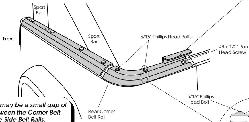
**Note:** There may be a small gap of +/- 1/4" between the Corner Belt Rails and the Side Belt Rails.
