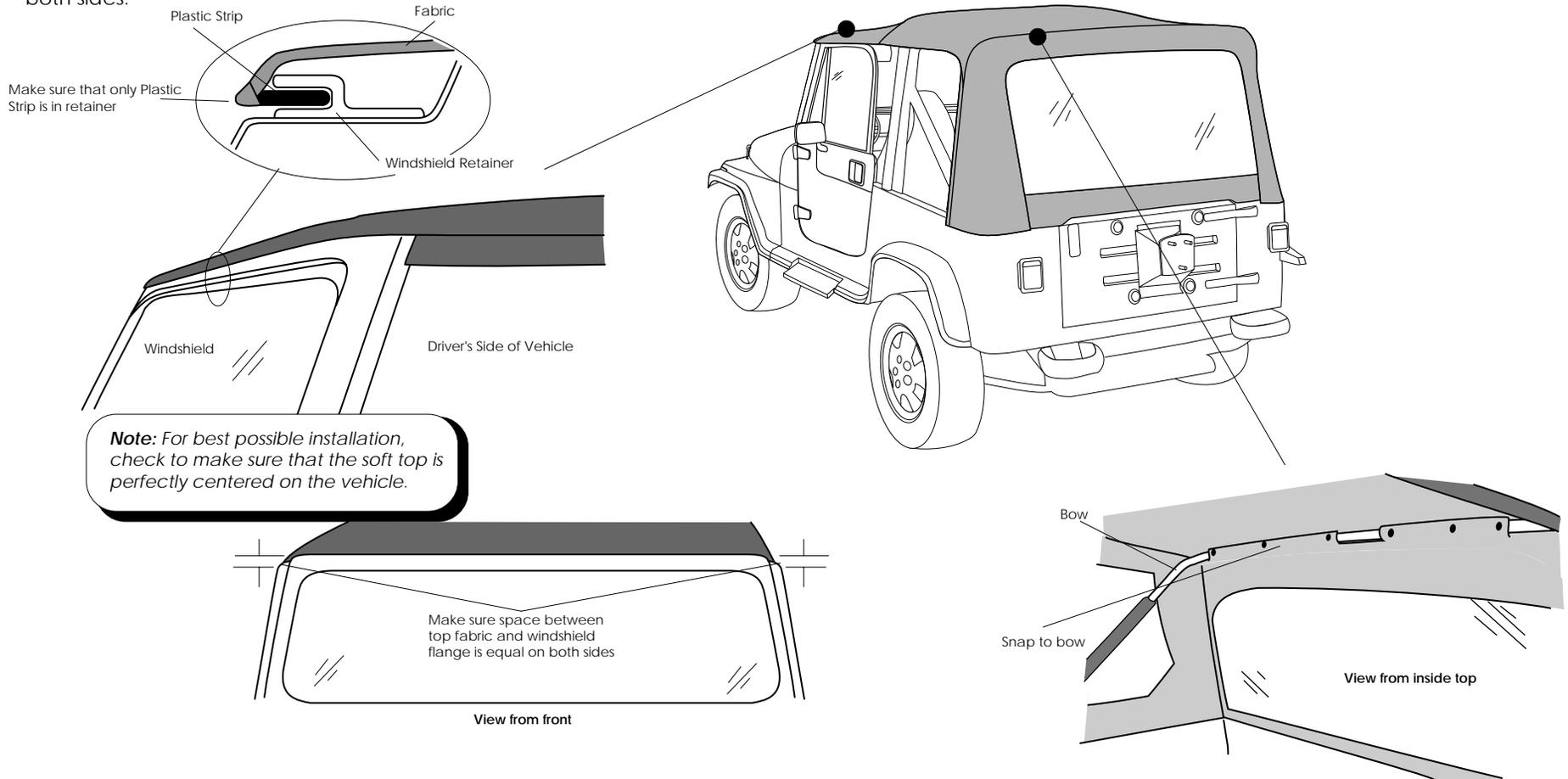
**Note:** If the snaps don't appear to line up, push the rear bow forward to relieve the pressure on the bow. This will allow the snaps to line up more easily.
