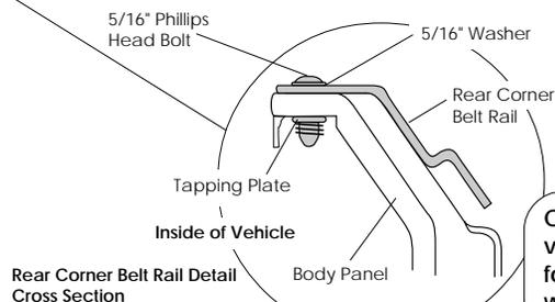
**Caution:** When drilling in the top edge of the vehicle body, check underneath for wiring for the rear lights. Pull the wiring out of the way before drilling.
