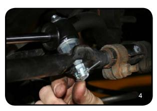
4. Insert new sleeve bushings into the new steering stabilizer shock, make sure you use ones that fit your factory hardware. If tight, tap them in with a hammer. (Photo #5,6,)
