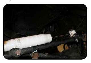
Install the new mounting pin into the steering stabilizer using the new nut and washers supplied and torque to 35 ft-lbs (photo #2)
