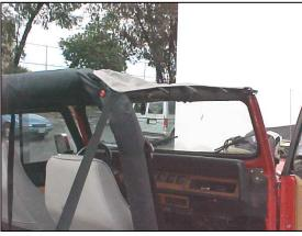
4. Pull the straps under the central roll bar through the Side Loops #1, then pull the straps towards the rear of the vehicle and insert through the Rear Loops #2 (Figures 5 & 6). Attach the strap to the mating buckle #3 (Figures 6 & 7).
