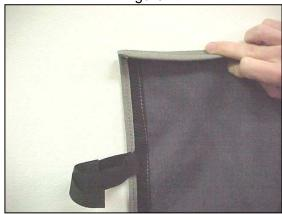
2. Place the Brief on top of Jeep. Insert folded edge into Windshield Channel, working from one side of vehicle to the other (Figures 2 & 3).
