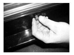
5. To mark the three bottom holes, stick a black marker through each hole and mark the vehicle making sure the mark is aligned vertically with the hole. Remove the rocker panels after the three bottom holes are marked. Use a center punch to mark each bottom hole so that from inside the vehicle, you can tell where the hole will be located. Before drilling, pull carpeting back and remove anything that might get in the way of the drill. Drill the three bottom holes to 7/16".
