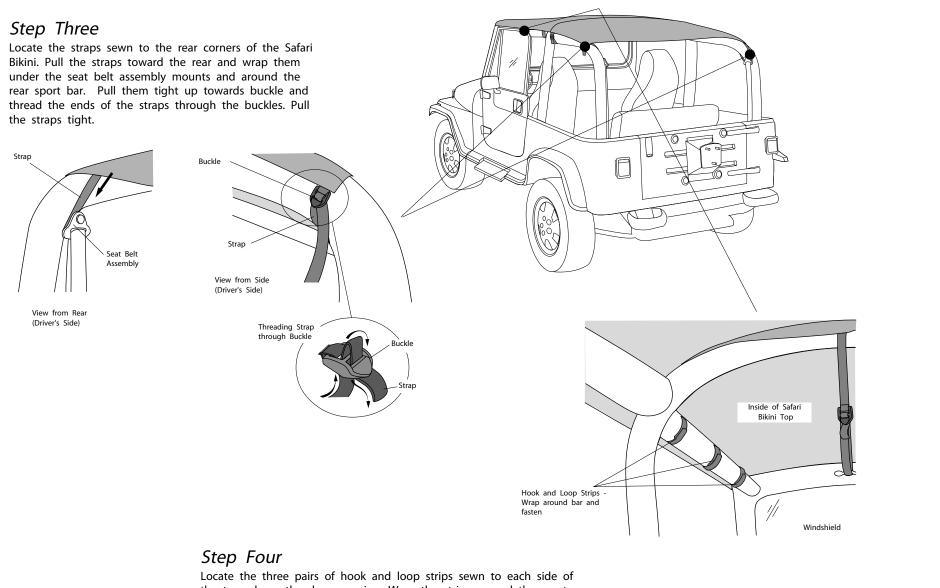
Locate the three pairs of hook and loop strips sewn to each side of the top, above the door opening. Wrap the strips around the sport bar and fasten them to each other. Make sure that all the hook and loop is as tight as possible.
