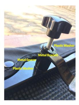
4. Place the header over the windshield insulation rubber. Adjust the positioning so the header is situated in the center of the windshield and on the rubber weather stripping along the top of the windshield. Lightly secure into position by having the metal bracket over the mounting loop on the windshield as shown in the photo below.
