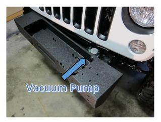
Cut away the vacuum pump bracket portion closest to the bumper. You can use any metal cutting tool to do this job (grinder, Sawzall, etc.).
