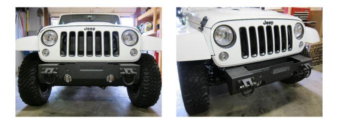
**NOTE:** If installing Rugged Ridge bumper ends to this modular bumper, do so before installing the bumper to the Jeep.
