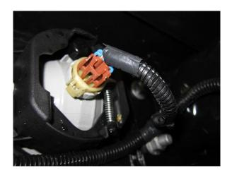
The full wiring harness runs the width of the Jeep and is clipped in place with 4 plastic push clips. Pull these from the steel bumper reinforcement.
