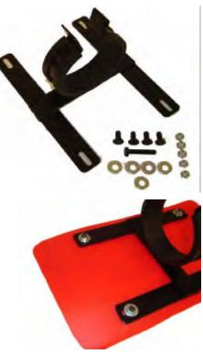
Step (2) Press license plate holder over the the front tube bumper as shown.Center license plate holder and secure it in place with (1) 1/4" x 1 1/2", (1) 1/4" flat washer, and (1) 1/4" nut.
