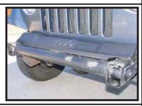
Step (2) Position the new front bumper up to the frame and line up the holes to factory mounting locations. Using the stock bolts and supplied flat washers secure bumper to vehicle. Be sure to use all hardware supplied and tighten all bolts.
