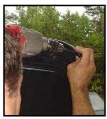
**Step 7:** After holes have been drilled using the 7/64" bit insert screws to secure Hood Armor to vehicle using a Phillips head screwdriver.
