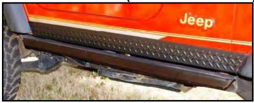
**Step 16:** Remove the two fender flare extensions from the body. Extensions are held in place by three bolts located outside of the Jeep® and are assessable from underneath the flare extensions.
