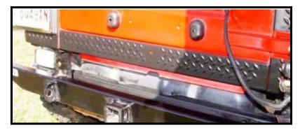
**Step 21:** Remove lower tire bump stop if so equipped.
