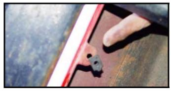
**Step 20:** Position armor onto lower side rocker panels. Make sure that it is evenly spaced before applying any pressure to armor. When satisfied with placement apply pressure to all areas to properly secure armor to vehicle. Secure bottom of rocker guards with hardware supplied.
