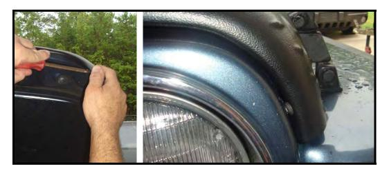
When properly installed the retaining screws should just be visible inside of the vehicle hood line and not interfere with the closing or locking of the hood.
