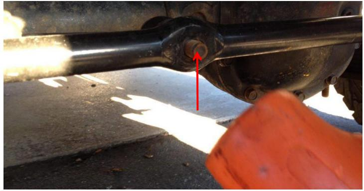
5. Remove the bolt securing the left side of the steering stabilizer, using a  $\frac{3}{4}$ " socket and 3/8ths ratchet. You're going to be reusing the old bolt for the new stabilizer.
