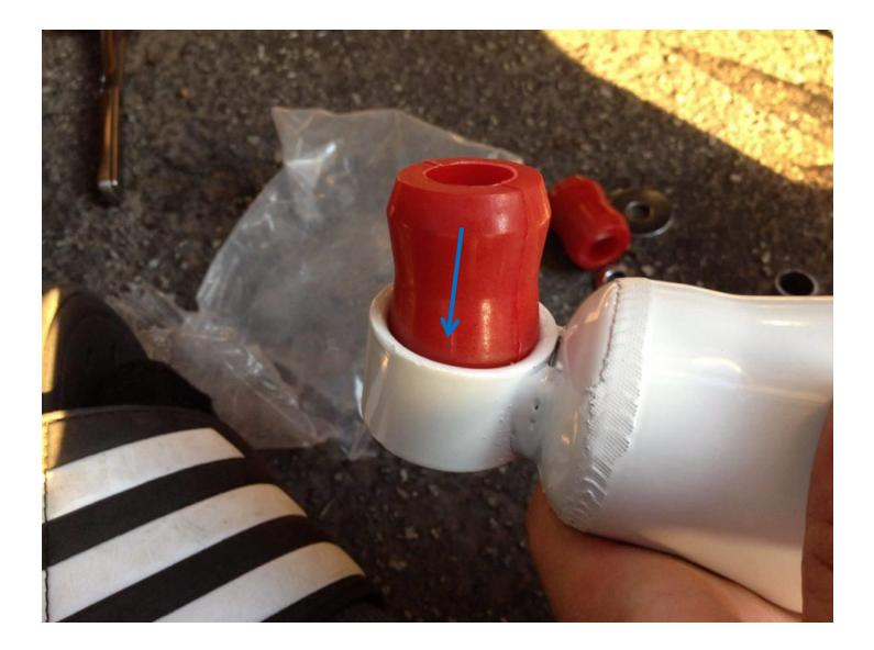
7. Next install the metal insert into the end of the stabilizer that uses the long  $\frac{3}{4}$ "-head bolt (not the one that bolts into the tie rod).
