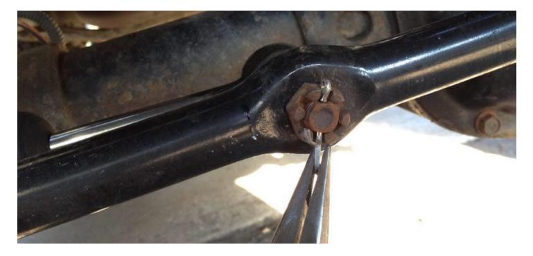
3. Remove castle nut. And smack out the stud with a rubber hammer. Be sure to hit the stud straight on and not too hard. If it's rusted in there, spray some PB blaster to break up the rust.
