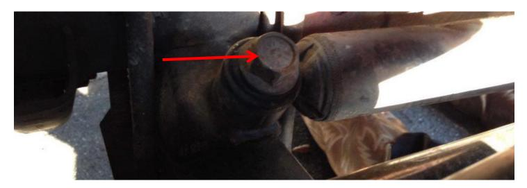
6. Now install the rubber bushings into both ends of the new Skyjacker steering stabilizer. Push the bushing through far enough so that it's an even amount of material on both sides. I recommend using silicone spray if it gets tough to push them in.
