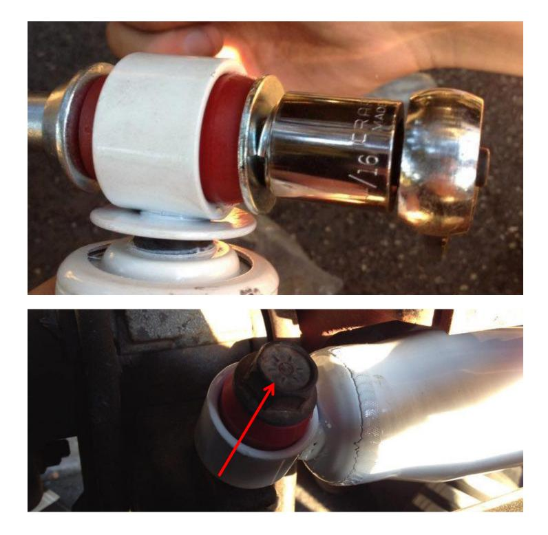
10. Next tighten down the nut holding the right side of the stabilizer onto the tie rod, using a ¾" 3/8ths socket, and a 3/8ths ratchet. Don't forget to install the sticker that comes with the new steering stabilizer, if you choose to.
