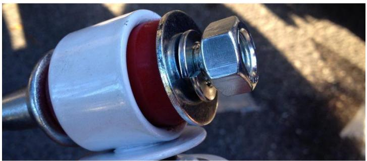
9. Tighten down the nut keeping the washers in place with an 11/16ths 3/8ths socket and a 3/8ths ratchet. Tighten down the nut until it fits snug against the red bushing. Then tighten down the bolt a quarter turn past snug, securing the left side of the stabilizer, using a  $\frac{3}{7}$  3/8ths socket and 3/8ths ratchet.
