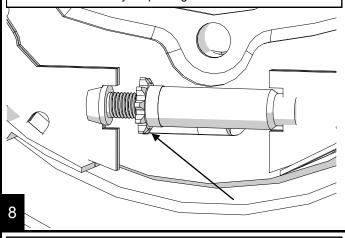
Non– C-clip applications– Install the new retaining plate and preload spacer on the axle shaft. Note: the orientation of the preload spacer is axle dependent.
