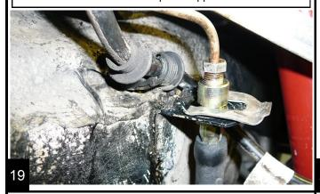
Install the emergency cable onto the lever at the mounting plate. TJ Wranglers order Tera part #TL869 for proper cables.
