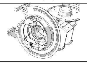
Adjust the internal drum brake with the adjuster until there is just enough room for the rotor to slide over the shoes. This will set your parking brake tension.
