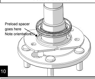
Press the new bearing and retaining collar onto the axle shaft.
