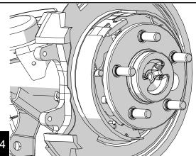
Install and tighten the nuts onto the retainer bolts through the access holes in the axle shaft and install the brake rotor.
