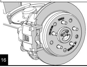
Install new brake hoses using new copper washers on the supplied banjo bolt. Install one copper washer onto the banjo bolt, slide the female end of the brake line onto the bolt, install another copper washer and install onto the caliper.
