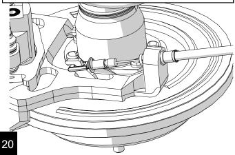
Reinstall tires torqueing lug nuts to 110 ft-lbs. Set the vehicle on the ground. Attach the emergency brake cables to the bracket under the body.
