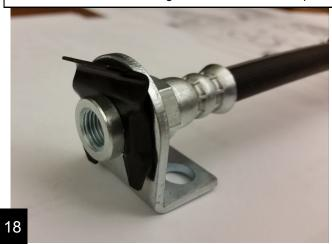
Connect the hard brake lines to the new soft lines and bleed the brakes starting with the passenger side then the drivers side. Note: You will need to purchase shorter metal lines from an auto parts supplier.
