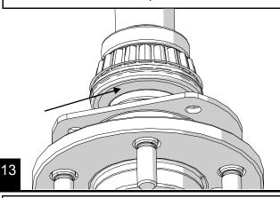
Carefully slide the axle in the rest of the way into the housing.
