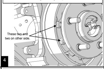
Remove the backing plate and wipe the bearing pocket surface clean of grease and contaminants.
