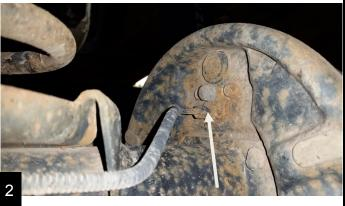
C-clip axle removal—Remove differential cover, unbolt the cross pin with an 8mm or 1/4" wrench and remove it from the carrier. Push the axles in about 1/2 inch to remove the C-clips. Remove C-clips and pull the axles from the housing.
