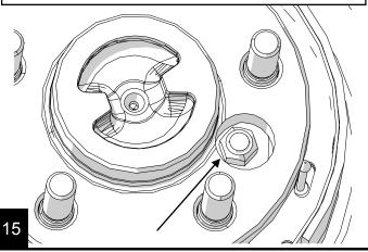
Install the rotor then install the brake pads into the caliper with the bleeder in the highest position. Note: install the inside pad first. Use the two supplied 8mm bolts, install the caliper onto the mounting plate. Torque to 11 ft-lbs.
