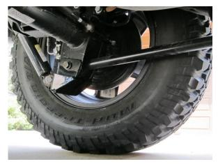
**CAUTION:** As with all steering and suspension components. After driving for a few hundred miles, be sure to re-inspect bolts, and re-tighten to 130 ft. lbs. if necessary.
