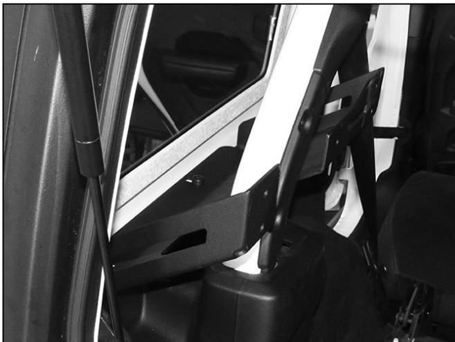
(Fig 3) Reuse (2) factory bolts to attach driver/left Side Panel to inside of top. Repeat to install the remaining passenger/right Side Panel
