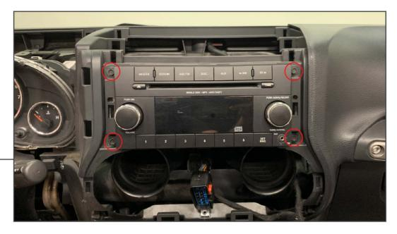
Remove the vehicles dash bezel to access the screws securing the radio to the vehicle. Using a 7mm socket, remove the (4) screws.
