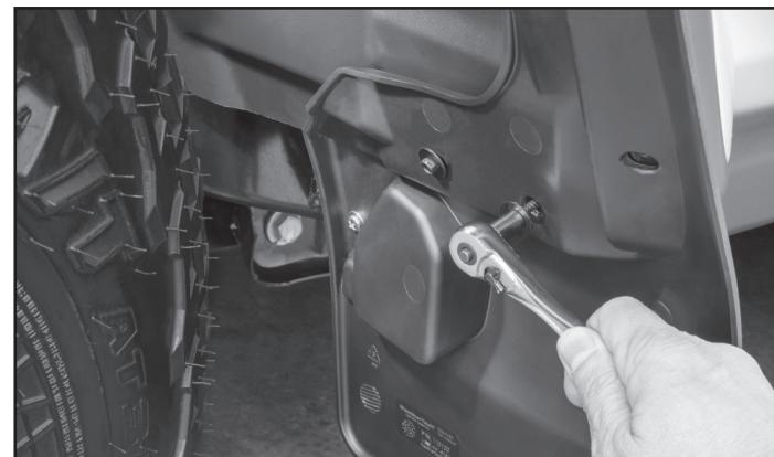
**10** Take (2) two supplied hex head screws from parts kit 48MF581 and install through the (2) two holes in the MudFlap as shown with the ratchet and appropriate socket to a loose fit.
