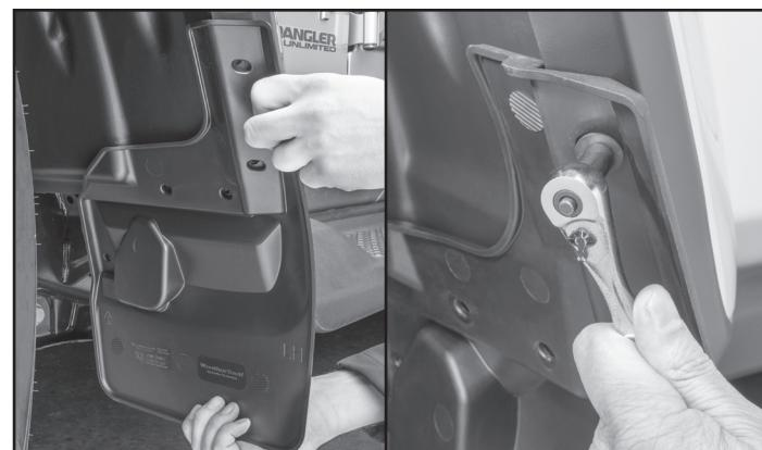
**8** Place the MudFlap marked, "LH," up to the fender and align with the corresponding holes. Then, take (1) one supplied hex head screw from parts kit 48MF583 and install through the top hole in the MudFlap with a ratchet and appropriate socket and loosely tighten.
