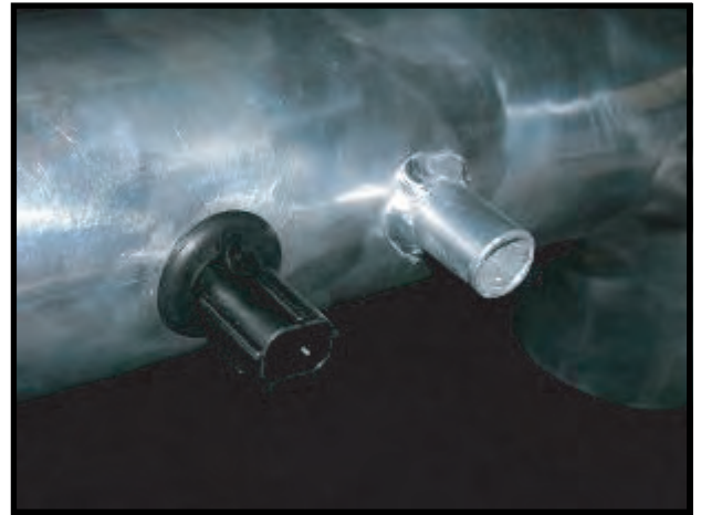
Sensor and Grommet installed in Intake Tube
