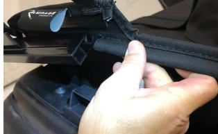
Tuck plastic strip into belt rail of vehicle body. It works best to start from the front and work your way back towards the rear.
