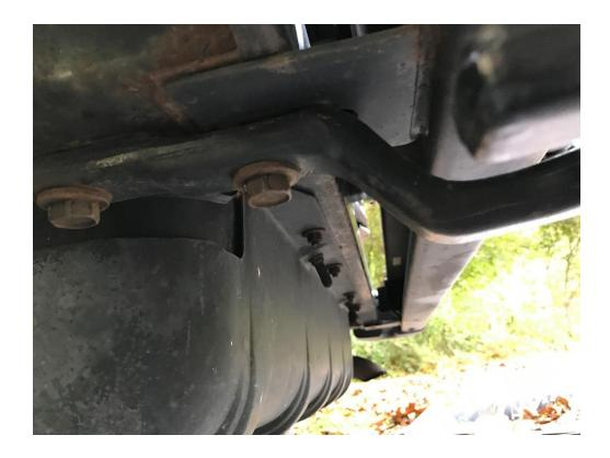
3. Using a 3/4" wrench, remove the bolts connecting the bumper to the crossmember (2 bolts on each side of bumper). Remove stock bumper from frame. \*Note: Stock bumper hardware will not be reused.
