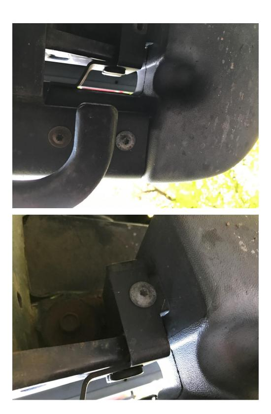
2. Remove the bolts which tie the bumper to the frame (1 bolt on the right side, 2 bolts on the left side, which run through the stock tow hook). \*Note: the stock tow hook will not be reinstalled
