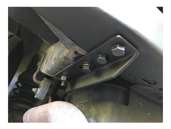
7. Fully tighten all nuts and bolts to complete installation.
