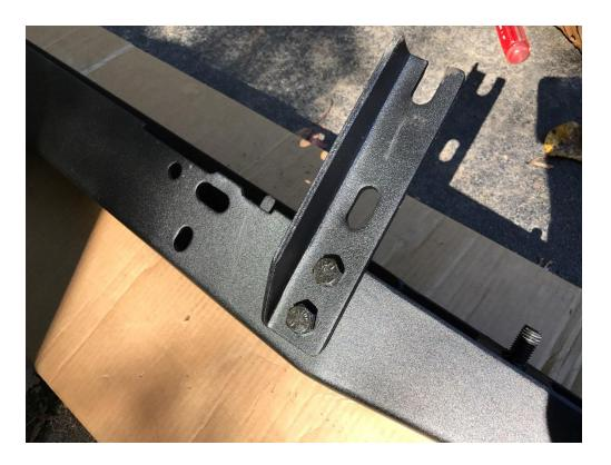
5. Mount bumper on the jeep by inserting the welded on bolts (2 on each side) into the holes on either end of the crossmember. Secure the bumper to the crossmember with included hex head bolts, flat washers, and nyloc nuts. \*Note: do not fully tighten these nuts
