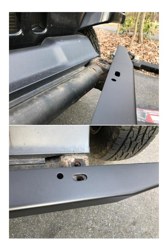
3. The new bumper uses only the front hole for installation. If your original factory bumper was equipped with tow hooks, place one of the included 1" washers between the bumper and tow hook prior to installation as shown below.
