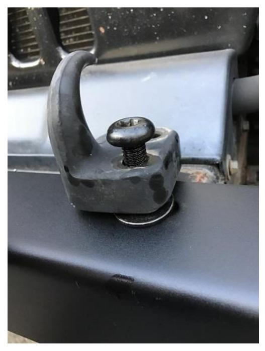
4. Reinstall a total of four bolts, one on each side of the top of the bumper, and one on each side of the bottom (bottom shown below). If equipped with tow hooks, reinstall all six bolts.
