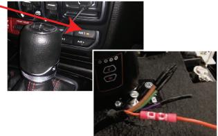
Step 19. If your JL/JT does not have these aux switches you can tap into the vehicle's Passenger Inline Fender Light Wire Harness Adaptor ONLY if you have headlights connected and no other RGB accenting lights connected to this Bluetooth RGB controller. Adding more RGB accenting lights will overload the circuit and the computer will shut that circuit off.
