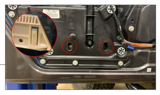
Ensure the window is all the way in the down position, using a razor knife carefully cut out the window retaining clip access plugs. This will expose the window retaining clips.
