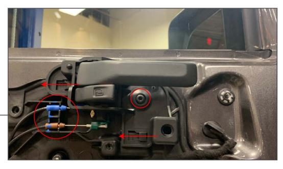
Unscrew the T30 Torx screw from the door handle. Then, slide the door handle back and unclip the door latch cables.
