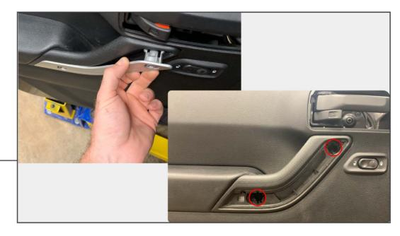
Using a soft pry tool, remove the door panel accent. Then, remove the (2) Phillips head screws
