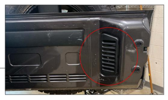
Tailgate Handle Install: Begin by opening the tailgate to access the interior panel.
