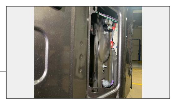
Using a 8mm socket, remove the (2) fasteners securing the handle to the vehicle.
