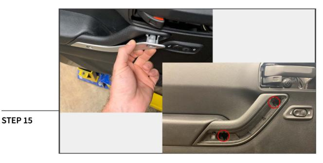
Using a soft pry tool, remove the door panel accent. Then, remove the (2) Phillips head screws
