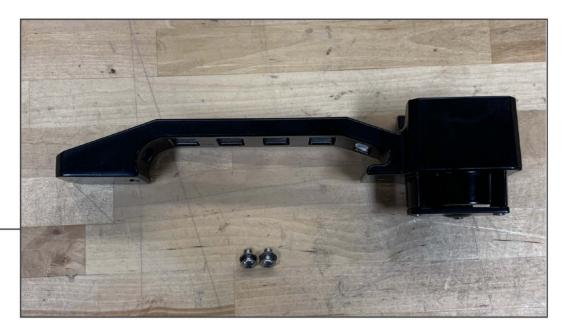
Install the door handle to the vehicle using the supplied M5 hardware.
