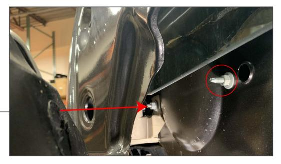
Using a deep 8mm socket, remove (2) nuts securing the door handle to the vehicle.
