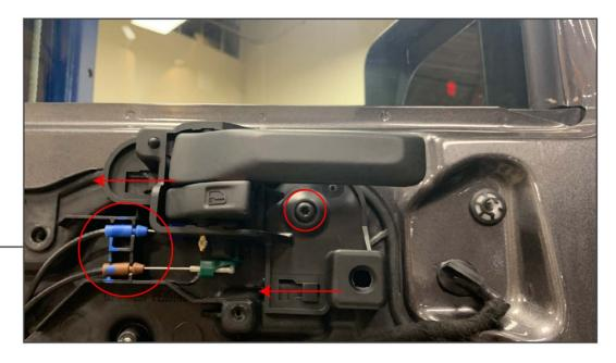
Unscrew the T30 Torx screw from the door handle. Then, slide the door handle back and unclip the door latch cables.
