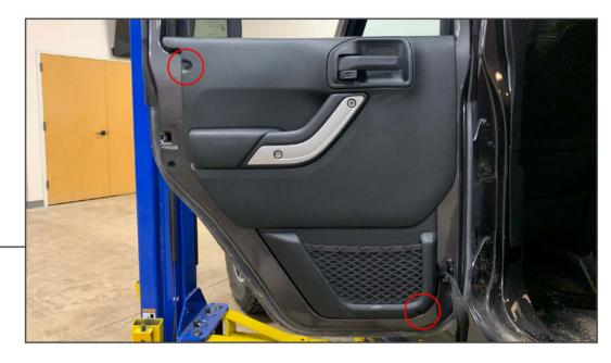
**Rear Door Installation:** Start by rolling the window all the way down. Then, using a T20 Torx bit, remove the (2) screws circled above.
