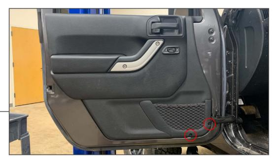
**Front Door Installation:** Start by rolling the window all the way down. Then, using a T20 Torx bit, remove the (2) screws circled above.
