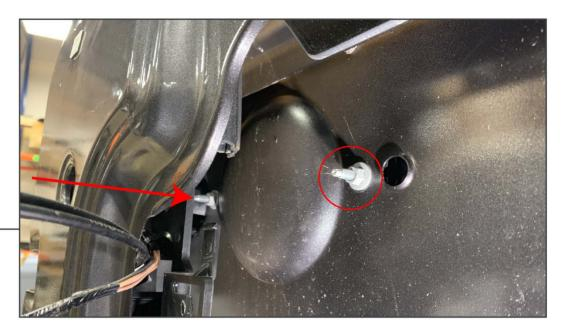
Using a deep 8mm socket, remove (2) nuts securing the door handle to the vehicle.
