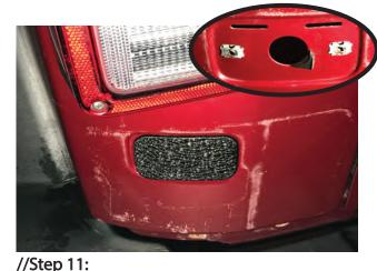
Remove the (2) screw inserts from the vehicle. Then clean the surface with isopropyl alcohol. Peel double sided tape from the delete plate and stick to vehicle. Once delete plate is installed, installation is complete.
