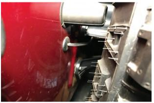
//Step 6: Route the LED wiring through the center cap hole on the wheel and through the spare tire mount. Run the wiring through the grommet in the tailgate.
