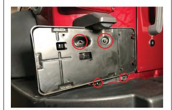
//Step 9: Remove the original license plate mount using a 7mm socket and remove the (4) screws.
