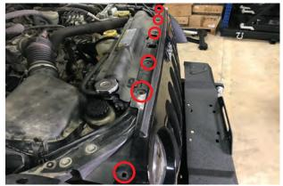
// Step 1: Using a panel removal tool, remove (6) plastic push clips.
