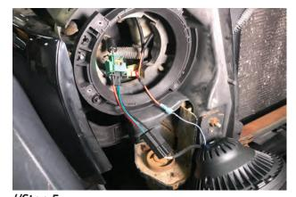
//Step 5: Once the harness has been wired, plug the harness into the headlight, as well as the original headlight harness into the new headlight.
