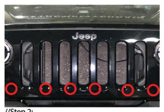
Pull firmly on the lower portion of the grille to unlatch (6) clips in the lower radiator support.
