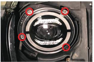
//Step 6: Install new headlight into original headlight bucket reusing (4) screws.
