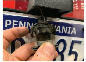
**Step 2:** Twist the bulb socket counterclockwise to remove it from the light housing.
