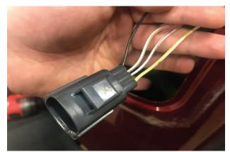
**//Step 6 (Wiring):** To wire the light to the vehicle, use the provided (3) Scotch-locks and tap into the vehicles wiring harness.
