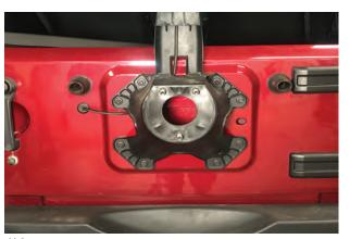
// Step 1: Begin by removing the spare tire off the mount using a 21mm socket and a breaker bar, and then remove the lug nuts. Lift the spare tire off the vehicle.
