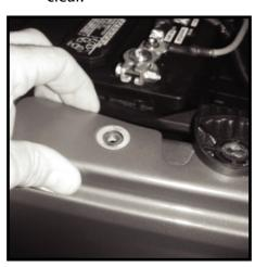
18 - Top cowl section of fender may be adhered to body.
