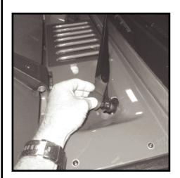
**103** - Slide 3/8" drain hose and 3/8" clamp to bottom of snorkel body.
