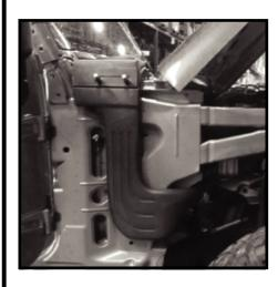
**93** - Tighten 3" clamp. Smooth and clean extra sealant from parts.
