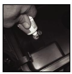
72 - Intsall (2) M8 nuts and (2) M8 flat washers to the underside of inner fender mounting plate. Add sealant if needed to insure a water tight seal.
