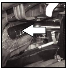
**90** - Slip main snorkel body and coupling over air tube as shown.
