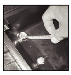
74 - Add sealant to inside of air box intake. Smooth sealant around intake lip and silicone elbow.
