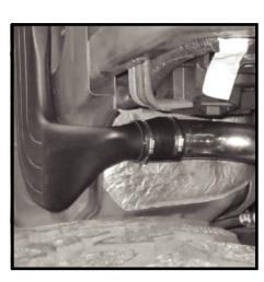
92 - Snorkel main body should rest in place as shown. Snorkel body should be fitted tight to inner frame. Make sure antenna cable is not hidden behind snorkel body.
