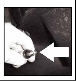
20 - Remove antenna mast from fender. With the assistance of another person pull fender away from vehicle just enough to disconnect antenna cable from fender.
