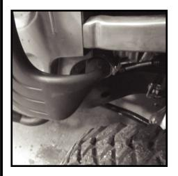
91 - Slide 3" clamp over coupling end. Inspect fit and alignment of main snorkel body to aluminum air tube.
