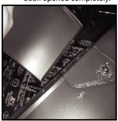
**26**- Cut out template from page 23. Place template over fender as shown.
