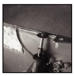
30- Using a Dremmel tool or angle grinder fitted with a metal cutoff wheel cut fender along marked lines. Cut should start in the middle of outer cut line (arrow). Cut should be 1/8" away from rolled edge. Cut in each direction towards 7/32" terminating holes (arrows). Eye protection should be worn.
