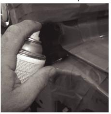
**83** - Make sure painting is done in a well ventilated area. Paint should not be applied in a windy environment. This will insure overspray does not fall onto vehicle. .
