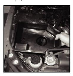
55 - If air box does not fit within 1/8" of rubber retainer grommets the top of the silicone air tube will need to be trimmed. Remove air box and elbow. If air box fits correctly proceed to step (57).
