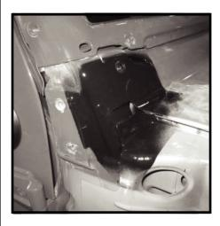
84 - Reinstall windshield bracket removed in step (2). Start and tighten the upper side M12 bolts and front M12 bolts as shownt.
