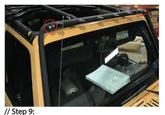
Install the upper windshield bar using (4) M10x1.50 35mm bolts, (8) M10 washers, (4) M10 lock washers, and (4) M10 nuts.
