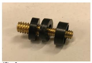
//Step 2: Assemble the bullet antenna fitting. Using (2) 7.5mm spacers, install them on the threaded fitting first. Then, install (1) 13mm spacer onto the threaded fitting.
