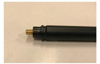
//Step 3: Once all spacers are on the fitting, thread the fitting onto the antenna. Tighten until secure.
