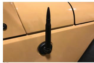
**//Step 4:**Thread antenna onto vehicle antenna base. Tighten until snug on vehicle. Once antenna is tight, installation is complete.
