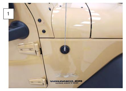
Locate the factory antenna and antenna base.
