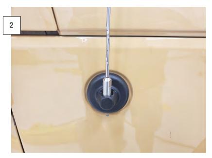
Carefully twist the antenna counter-clockwise to remove. Remove the factory antenna.
