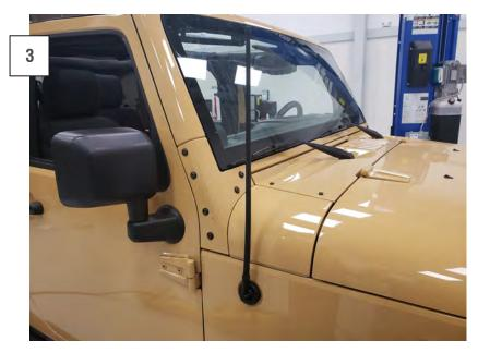
Install the new antenna by twisting it clockwise. Installation is now complete.
