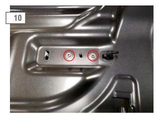
Remove the (2) 10mm nuts securing the windshield washer fluid squirter's on each side. Remove the squirter's from the hood. Transfer the squirter's to the new hood.
