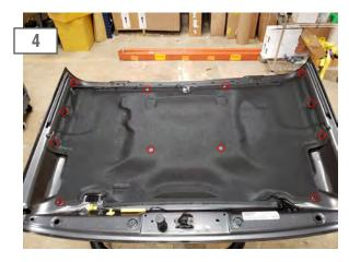
Using a trim panel removal tool, remove the (12) plastic push pins securing the hood liner to the hood. Remove the hood liner.
