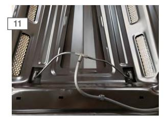
Install the factory windshield washer fluid hose line to the new hood. Trim to fit.
