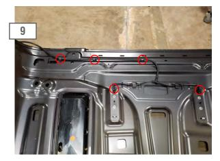
Using a trim panel removal tool, carefully pry up to release the windshield washer nozzle hose from the hood. Then disconnect the hose from the squirter's. Remove the hose from the factory hood.
