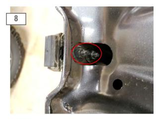
Remove the (2) 10mm nuts that hold the hood latch to the hood. Remove the latch from the hood. Transfer the hood latch to the new hood using the factory hardware. Do the same for the opposite side.
