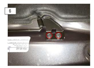
Remove the (2) 10mm bolts securing the hood prop rod to the factory hood. Remove the hood prop rod. Transfer the hood prop rod to the new hood using the factory hardware.
