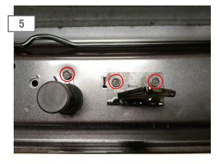
Remove the (2) 10mm hood latch bolts, and (1) 10mm hood stopper bolt. Remove both the hood latch and the hood stopper. Transfer both the hood latch and the hood stopper to the new hood using the factory hardware.
