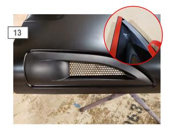
Using a isopropyl alcohol, clean the new hood where the hood bezels will be applied. Allow time to dry. Test fit the hood bezels to familiarize where they install. Remove the tape red tape backing on the hood bezels. Apply firm even pressure to the tapped surfaced areas to ensure proper adhesion.
