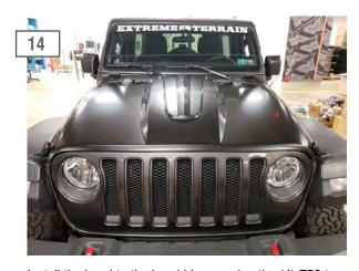
Install the hood to the hood hinges using the (4) T50 torx bolts. Be sure to align hood for proper open and closure. Reconnect the windshield washer hose line from Step 2. Installation is now complete.
