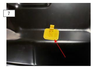
Using a trim panel removal tool, carefully remove the hood prop retainer clip. Transfer to the new hood.
