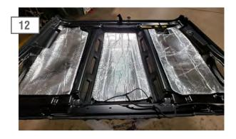
Using a isopropyl alcohol, clean the new hood where the heat shields will be applied. Peel the backing off the supplied heat shields. Install the supplied heat shields to the new hood by applying firm even pressure to the tapped surfaced areas to ensure proper adhesion.
