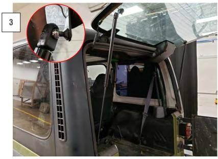
Carefully press the new support over the ball socket until it clips in place. Repeat this for the top and bottom of each support. Installation is now complete.
