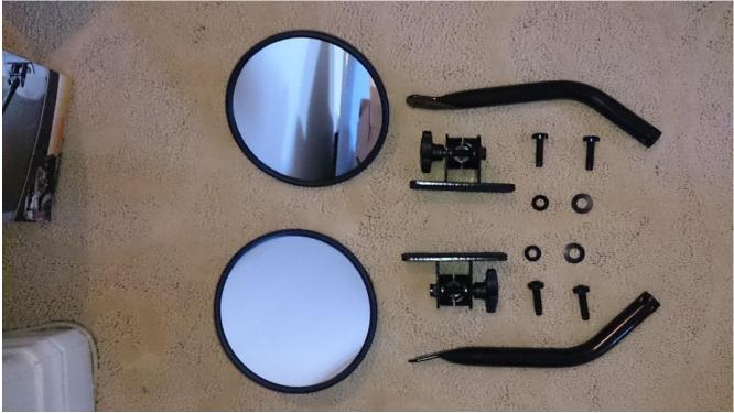
The two 5/16" bolts have been supplied for TJ & LJ Models. JK models will reuse the factory hardware.
