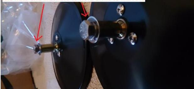
2. Locate the two upper bolts of the Windshield Frame and unscrew using T40 Torx Wrench.
