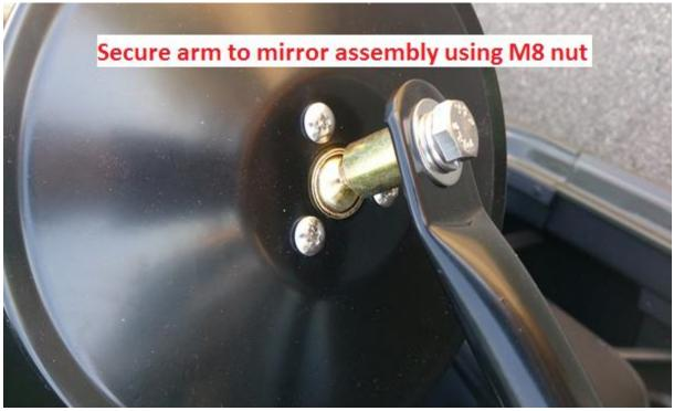
5. Using the Knob, Billet Bushing and freshly constructed mirror/arm assembly, secure the mirrors to the brackets on the windshield frame.
