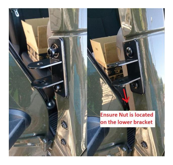
4. Next, set up the mirror by securing the arms to the mirror using the M8 bolts / washers as shown. The M8 Bolts will require a 13mm socket wrench to tighten.
