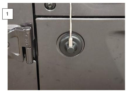
Remove the factory antenna rod. Wash the factory antenna mount with soap and water. Allow the antenna mount time to dry. \*\*Recommended: Wipe the mount down with isopropyl alcohol to ensure the cleanest surface possible.
