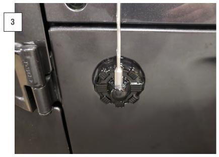
Reinstall the factory antenna rod. Installation is now complete.
